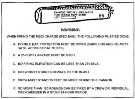
Figure 2-27. M203 propelling charge (red bag)
