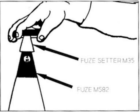
Figure 3-22. Fuze setter M35 on fuze M582
