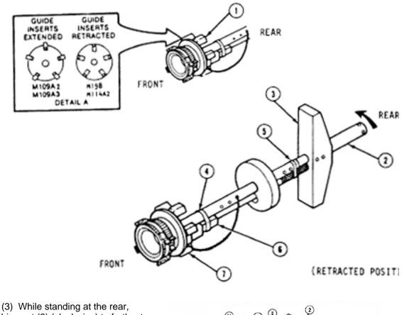
(3) While standing at the rear, loosen drive nut (2) (clockwise) to farthest white marks (forward mark).
