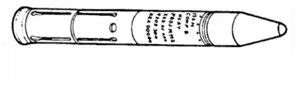
Figure 2-22. M712 (CLGP) projectile (fins and wings retracted)
