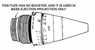
Figure 3-10. Fuze M565 mechanical time
