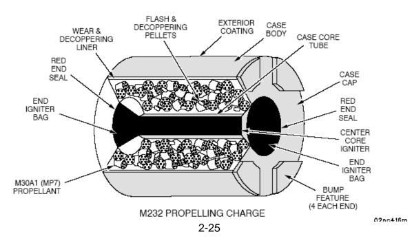
The M232 propelling charge is comprised of a tan-colored, coated,<br/>-based combustible case with black markings. This charge isnitrocellulose-<br/>bi-directional<br/>(can be loaded in either direction). Each end has four raised 1/8--inch bumps. The<br/>M232 is fired in increments of 3 through 5 for charges 3 through 5.
