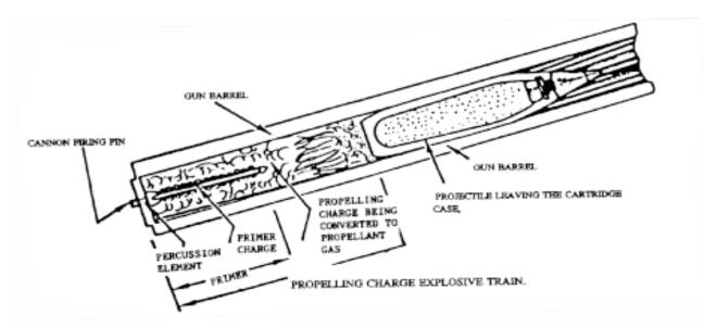
Figure 1-7b. Propelling charge explosive train upon firing
