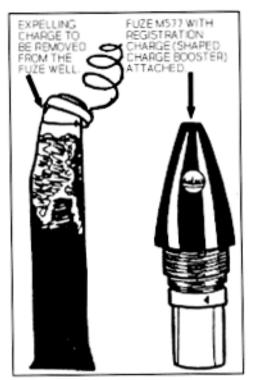
Figure 3-19. M577 fuze and booster charge
