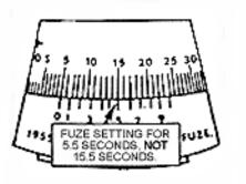
(2) Setting the fuze to safe. If the fuzed projectile is prepared for firing but is not fired, place the M63 fuze setter back on the fuze. Realign the S mark on Figure 3-16. the upper scale (MA on the M563 fuze) with the 0 mark on the vernier scale
