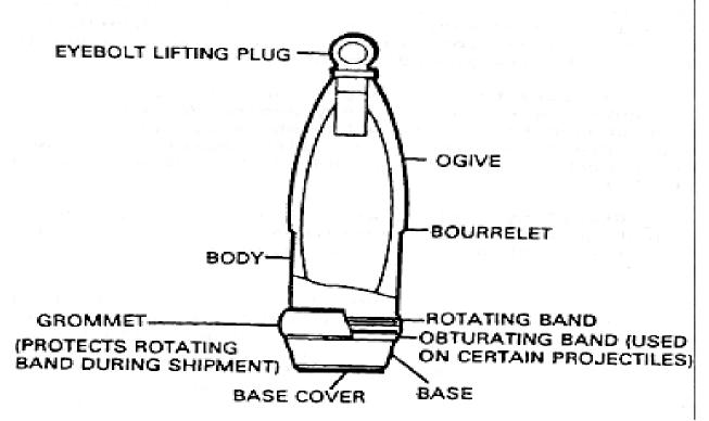
Figure 1-3. Exterior components of projectiles
