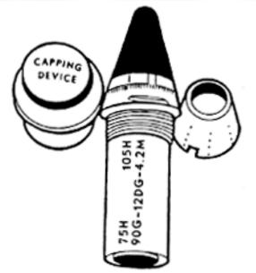
Figure 3-27. Capping device, M513 VT fuze, M5 desensitizing cap
