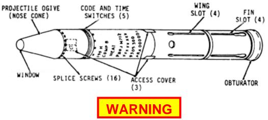
The M823 training projectile must not be fired. Such firing could be a hazard to personnel forward of the weapon.
