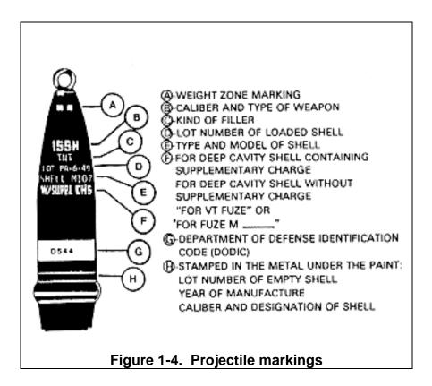
The next marking designates the kind of filler in the projectile. In Figures 1-4 and 1-5, this filler is TNT.
