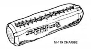
Figure 2-26. M119 propelling charge
