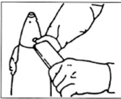
Figure 3-20. Using the M18 fuze wrench
