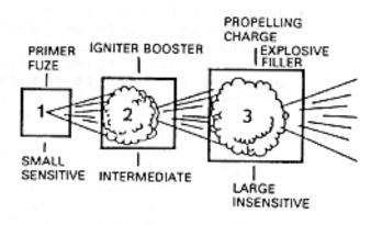
Figure 1-6. Explosive train principle
