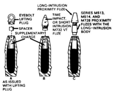
Figure 3-29. Deep cavity projectile with supplementary charge
