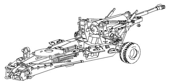
Figure 2-12. M198 howitzer in the towed position
