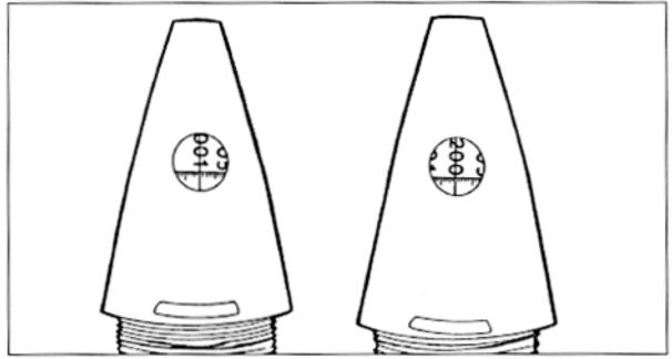
Figure 3-25. Start time setting and maximum time setting of fuze M577 or M582
