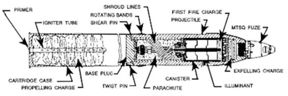
Figure 2-6. Illuminating projectile
