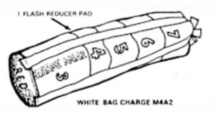
Figure 2-25. M4A2 propelling charge
