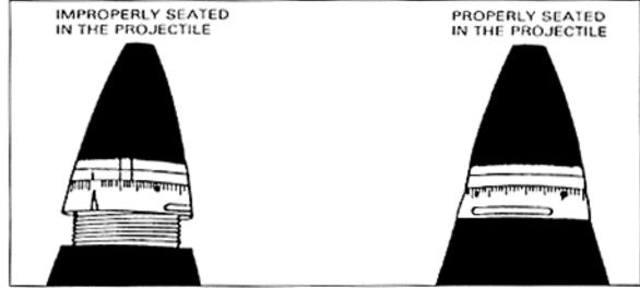
Figure 3-30. Left, improperly installed VT fuze; right, properly installed VT fuze 3-24
