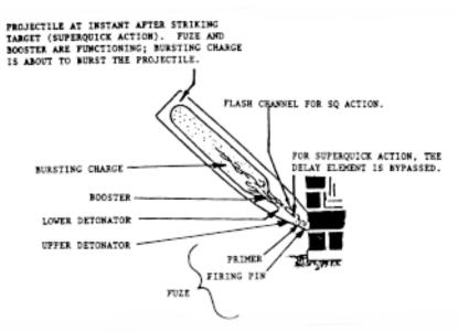
Figure 1-7c. Bursting charge explosive train on impact
