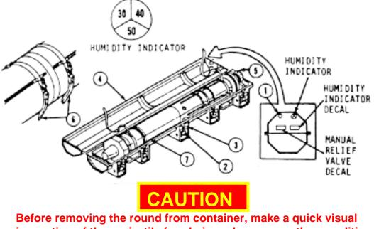
inspection of the projectile for obvious damage or other condition that would prevent use. If projectile appears not usable, replace lid and return to battalion maintenance.
