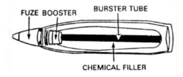
Figure 1-11. Bursting tube explosive train
