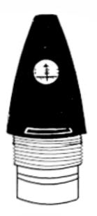
Figure 3-24. SQ/PD setting of fuze M577 or M582
