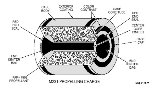
The M231 propelling charge is comprised of a green-colored, coated, nitrocellulose-based combustible case with black markings and black bands. This charge is bi-directional (can be loaded in either direction). The M231 is fired in increments of 1 or 2 for charges 1 and 2.
