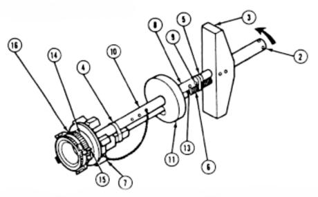
(1) Disengage locking pin (7) and compress telescoping shafts to retracted position.
