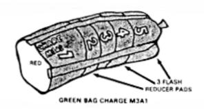
Figure 2-24- M3A1 propelling charge
